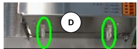
Fig. 18: TeleLite “Swing-Out” shelf connection cable guides
