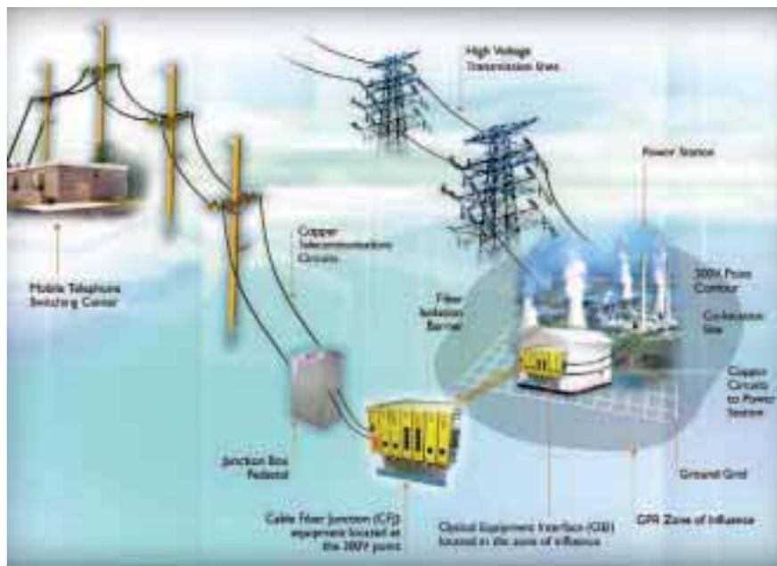
Figure 3: Fiber Isolation at a power station
